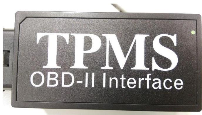
If the OBD II module displays a continuous red light, it indicates that the ID writing failed and you should turn off the car's ACC, disconnect the OBD II Module, plug it back and then turn on the ACC before a new attempt.
