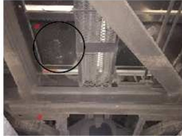
Fig 3. Antenna fixed on the bottom of the chassis.
