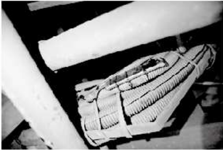
Fig 1. The antenna is tied to cable harness.
