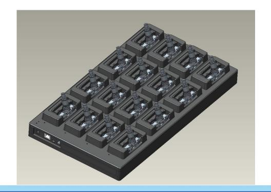
Choose the Program option in order to program 1 or more sensors. Make sure the sensor(s) are placed in the cradles and the latches are closed to ensure a proper contact between cradle pins and sensor pads.
