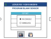
Select the programming mode with the arrow keys (see description below), then press the "OK" key to program.
